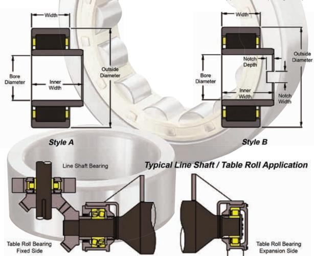
The table on the following page is a listing of Rollway's 5200 series cylindrical radial roller bearings that are used in these applications.
