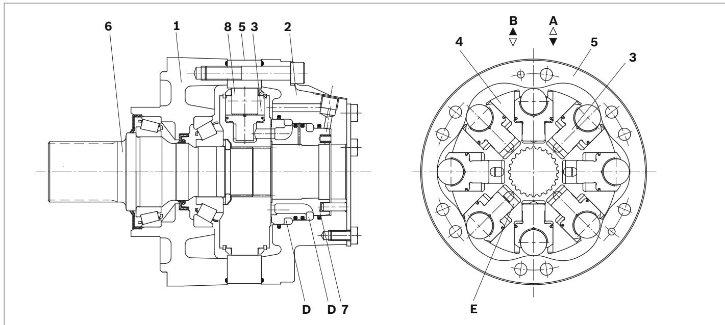
Hydraulic motors of the type MCR-D, MCR-E are radial piston motors with front case mounting and parallel shaft with key. MCR-D and MCR-E have the same type of rotary group and rear case assembly but differ in the front case mounting. These motors are intended for open or closed circuit operations as drive motors for various industrial applications.
